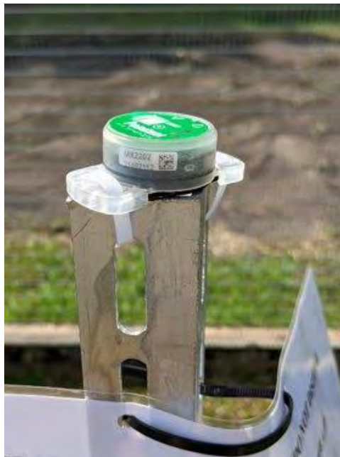
Figure 10.1 HOBOTRON MX2202 Temperature and Light Data Logger deployed during the baseline study.
