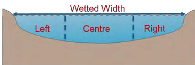
Figure 8.3 Calculation of cross-sectional area from the wetted width and averaged depth across the left, centre, and right stream portions.
