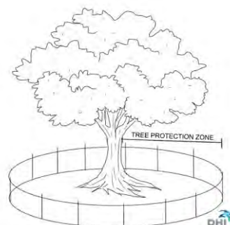
Figure 13.1 General guideline for minimum protection zone (radius) (NParks, 2023) and depiction of TPZ set up.
